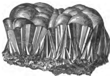
FIG. 64.—Piece of hæmatite, showing the nodular external form and the internal crystalline structure.
